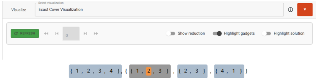
Figure 3.9: The D3 set template rendering an Exact Cover problem instance. The universal set \{1, 2, 3, 4\} is displayed alongside candidate subsets \{1, 2, 3\} , \{2, 3\} , and \{4, 1\} . Each set is rendered using curly brace notation, with nested elements displayed as individual labeled tiles. Both sets and their constituent elements are individually highlightable via the gadget system — selecting any set or element propagates the highlight to all semantically corresponding components across the reduction chain, consistent with the transitive map \Phi defined in Section 3.5.
